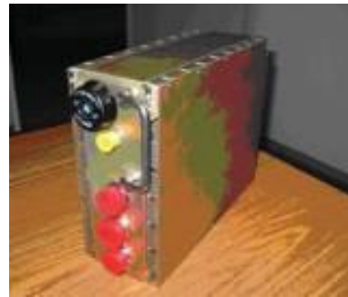
Control electronics chassis (in-process prior to paint)
